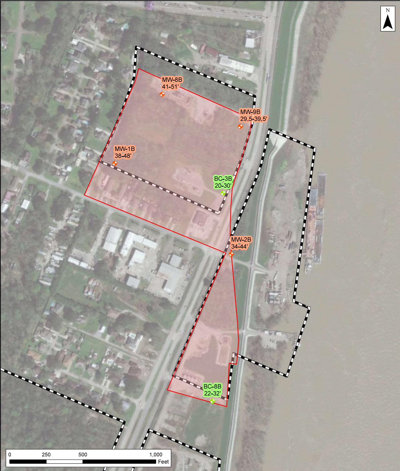
Figure 108 Proposed Wells for Groundwater Monitoring Hero Lands Company, L.L.C. vs. Chevron U.S.A. Inc., et al. Stella Oil & Gas Field Plaquemines Parish, Louisiana
