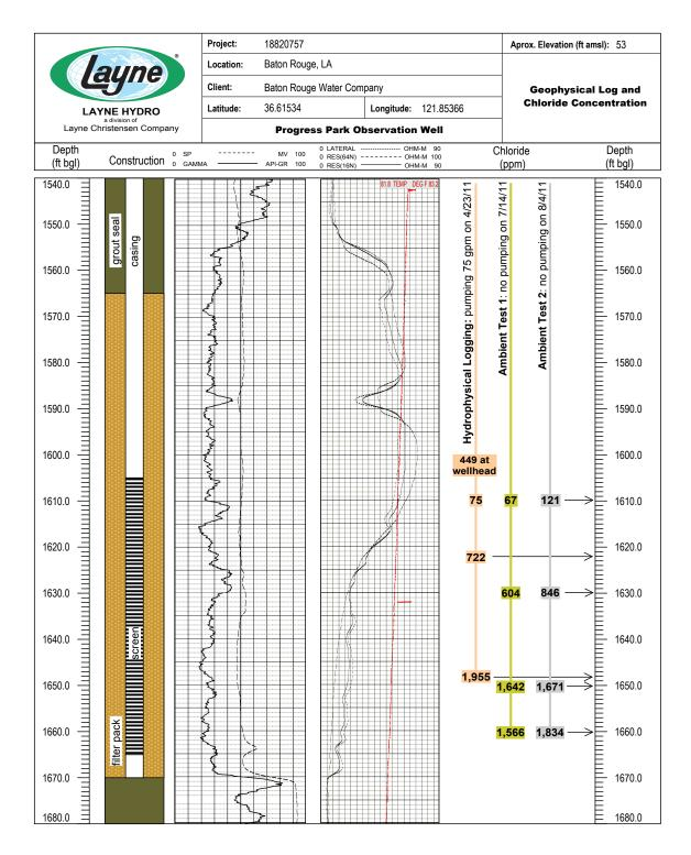
Figure 12: Chloride concentrations in the Progress Park observation well at discrete depths during active pumping and non-pumping conditions.
