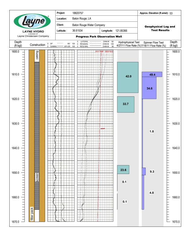
Figure 11: Results from flow testing the Progress Park observation well, including a hydrophysical logging test conducted on 4/27/11 while pumping 75 gpm and a spinner flowmeter test conducted on 7/18/11 while pumping 221 gpm.
