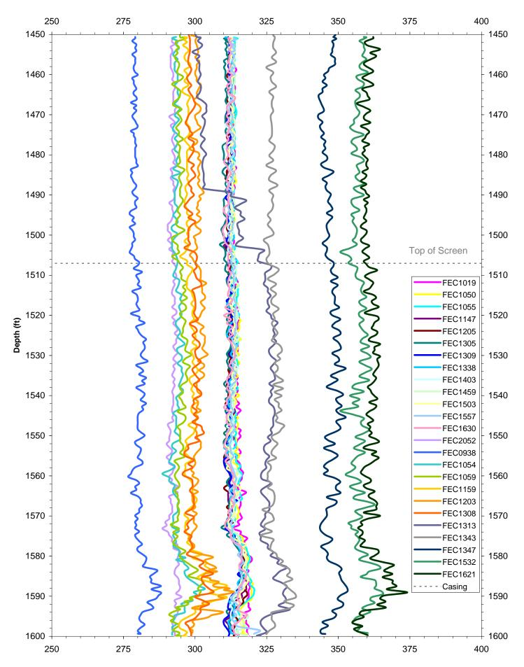
FIGURE Well 19:2. Summary of Fluid electrical Conductivity Logs During Pumping at 725 GPM;Wittman Hydro; BRWC; Baton Rouge, Louisiana; Wellbore: #19
