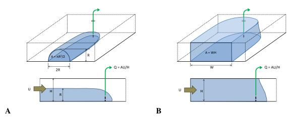
Figure 32: Conceptual sketches of the capture zones for a partially penetrating well of small discharge (A) and large discharge (B).
