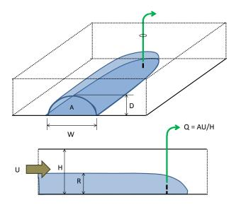
Figure 33: Capture zone for a partially penetrating well with small discharge in an anisotropic aquifer.
