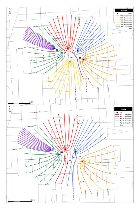
Figure 6: Capture zones of Lula wells with all wells pumping (A) and all wells pumping except Well 19 (B).
