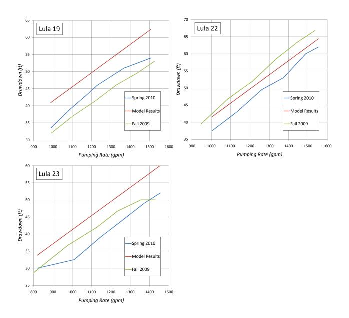
Figure 20: Comparison of drawdown from annual spring and fall well-testing with model results for BRWC wells.
