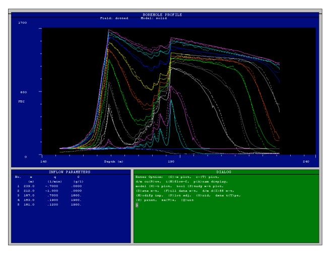
Figure 5. Concentration (= FEC) versus depth at a series of times for example application 4 – down flow. Figure is a BORE II screen-print after running option R.
