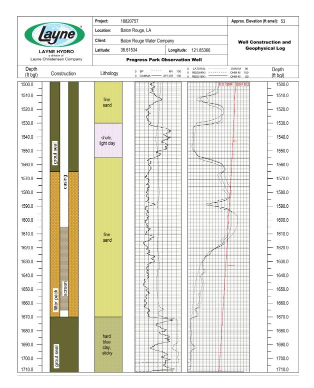
Figure 9: Comparison of lithology and geophysical log to the screened interval at the Progress Park observation well.
