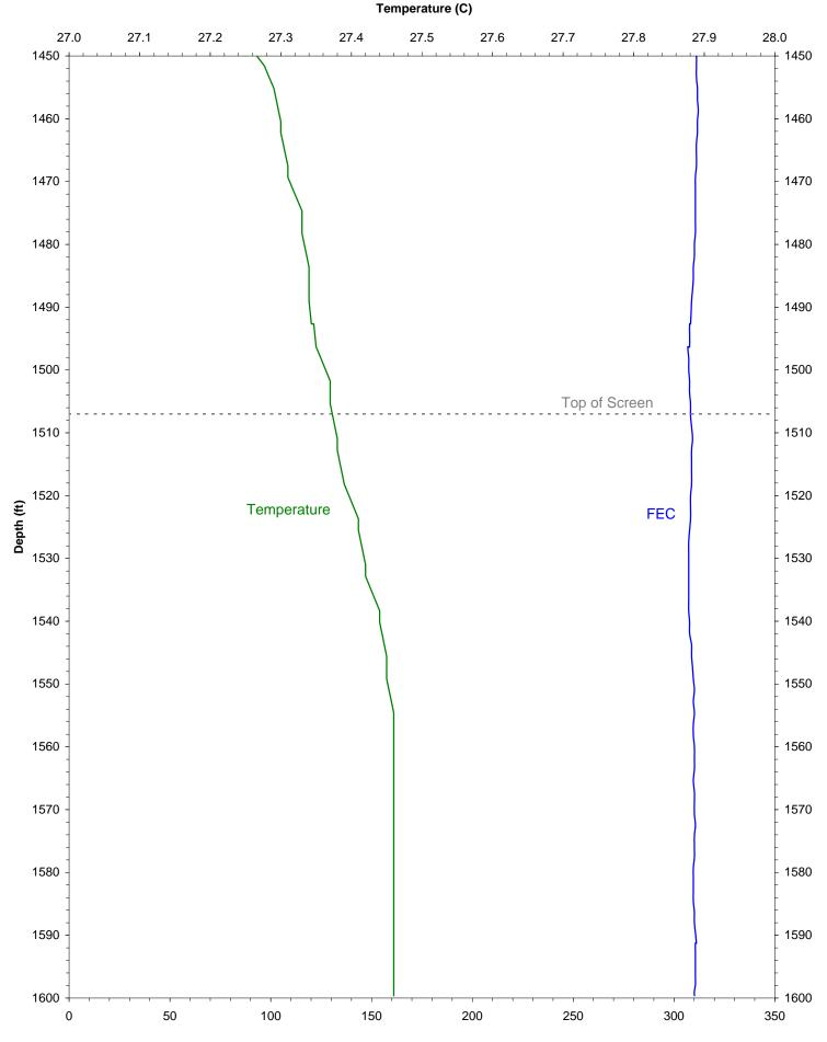
FIGURE Well 19:1. Ambient Temperature and Fluid Electrical Conductivity;Wittman Hydro; BRWC; Baton Rouge, Louisiana; Wellbore: #19
