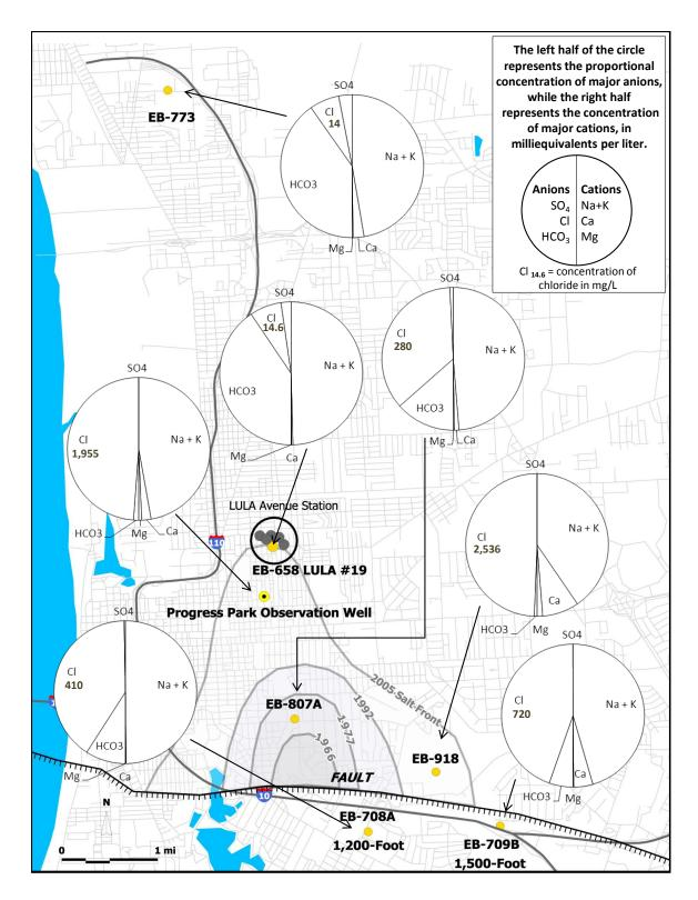
Figure 13: Comparison of general water-quality characteristics of saline water at Progress Park with new results from EB-918 and existing data from the 1,500-Foot and 1,200-Foot sands.
